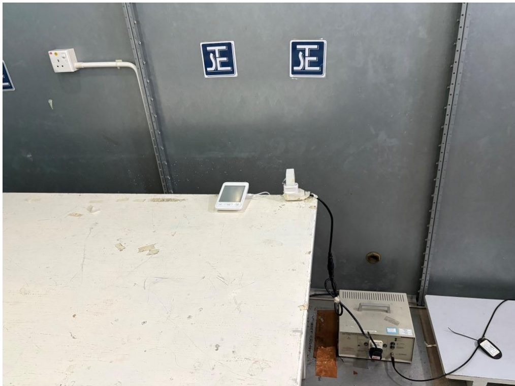
Conducted Emission Test Set Up
