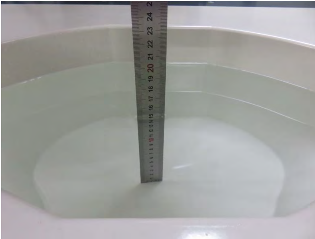
Photograph of the depth in the Body Phantom (2450MHz, 15.0cm depth)
