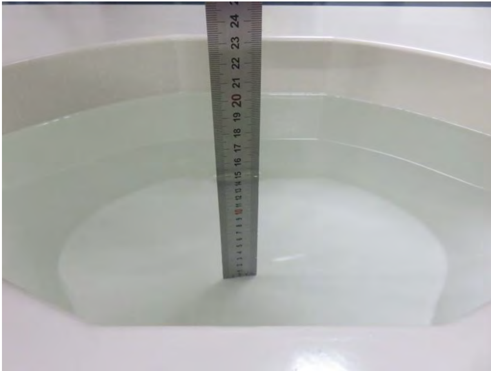
Photograph of the depth in the Body Phantom (1800MHz, 15.3cm depth)
