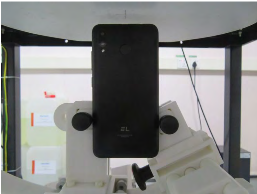
10mm body-worn Top Side Setup Photo (hotspot)
