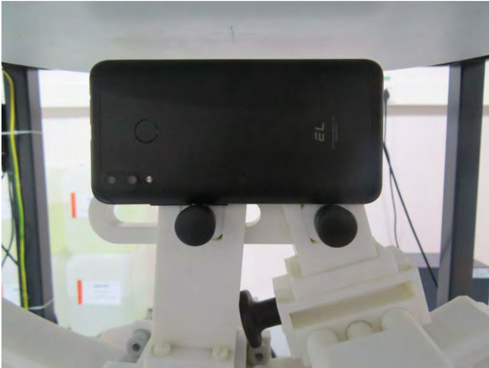
10mm body-worn Left Side Setup Photo(hotspot)
