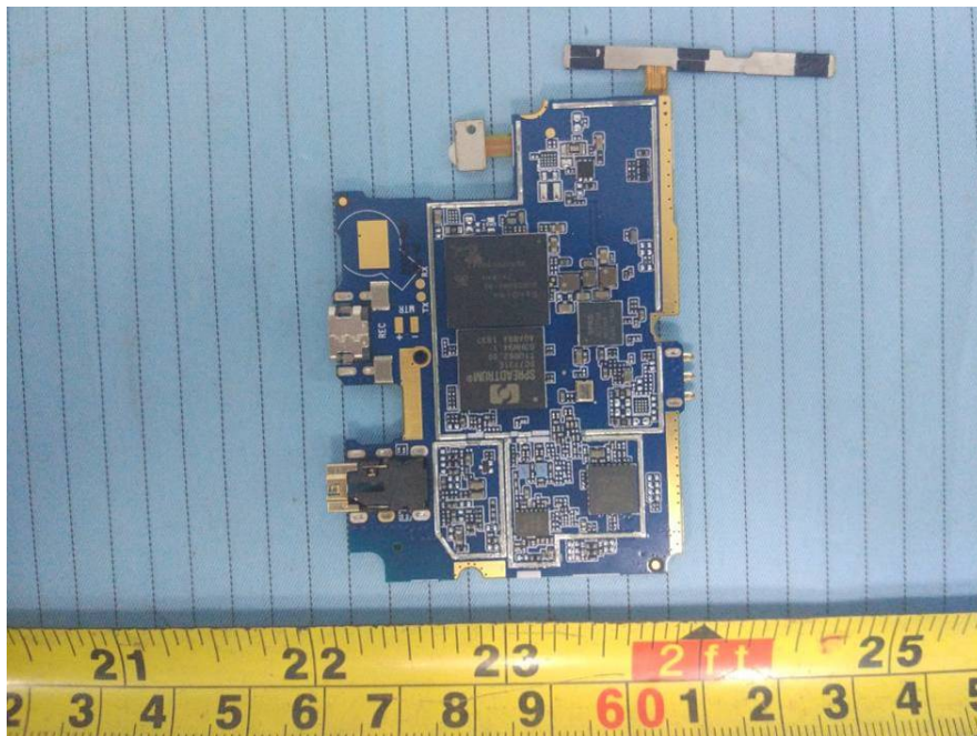
EUT – Main Board Bottom Shielding off View
