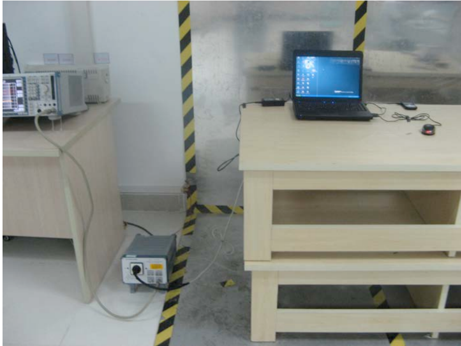
FCC LINE CONDUCTED EMISSION TEST SETUP
