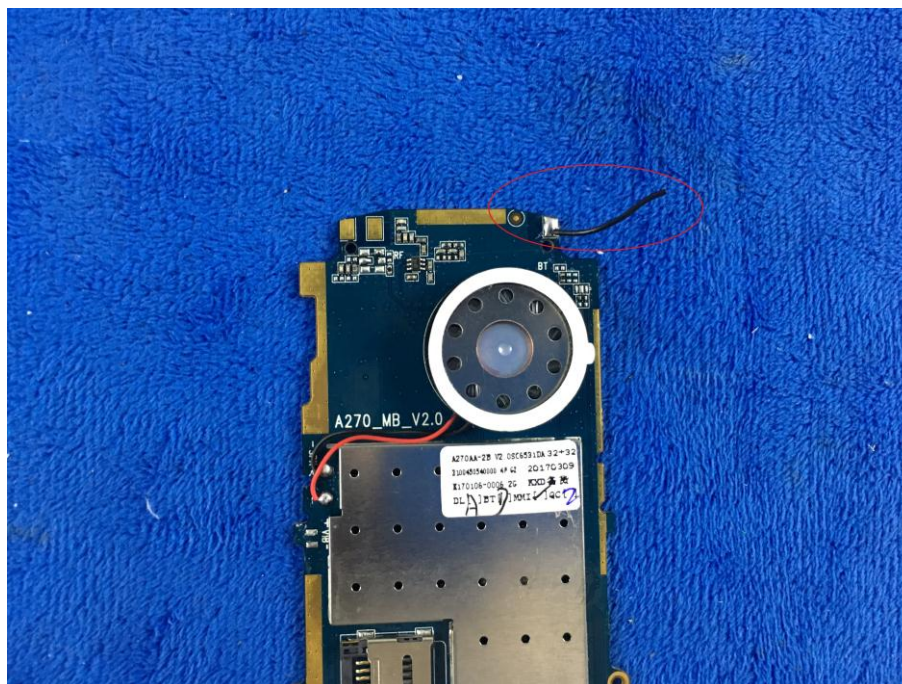
BT - Antenna View
