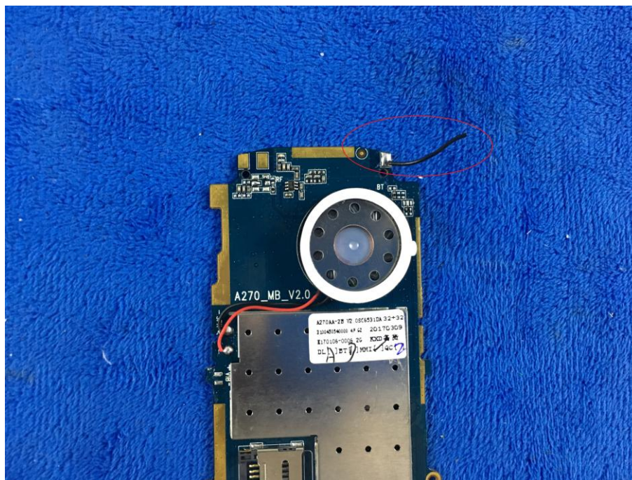
BT - Antenna View
