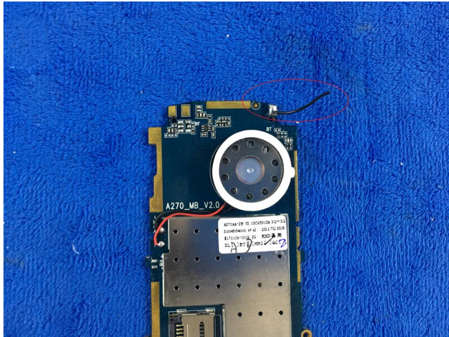
BT - Antenna View
