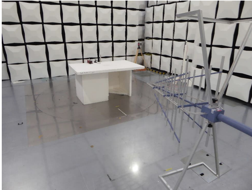
EUT tabletop Test setup semi anechoic chamber M276 Preliminary and final measurement 30 MHz - 1 GHz
