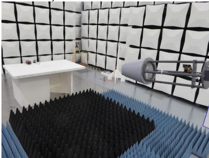
EUT tabletop Test setup semi anechoic chamber M276 Preliminary and final measurement 1 GHz – 18 GHz
