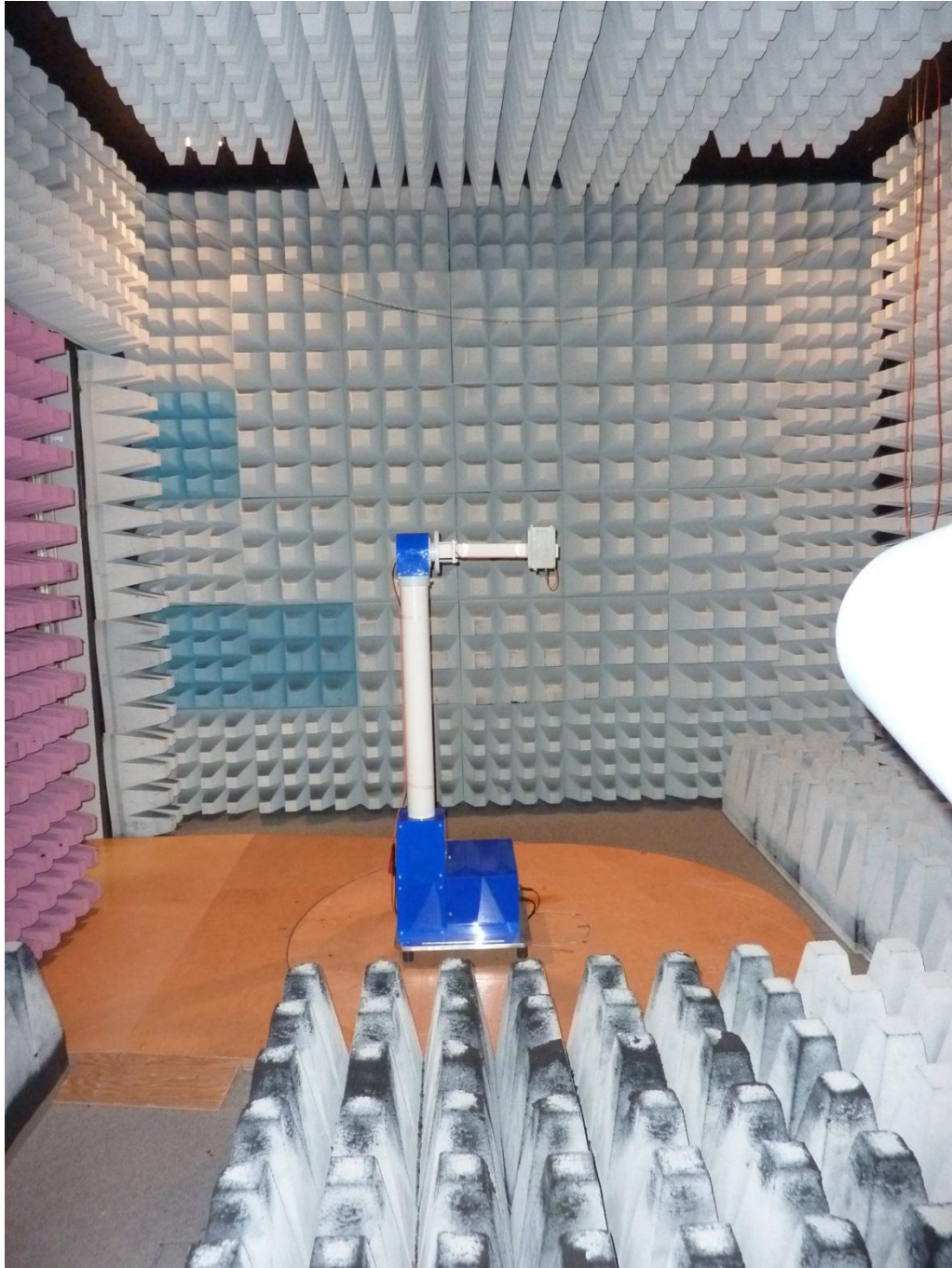
161597_8.JPG: ZONESCAN 820 Solar Alpha, test setup fully anechoic chamber
