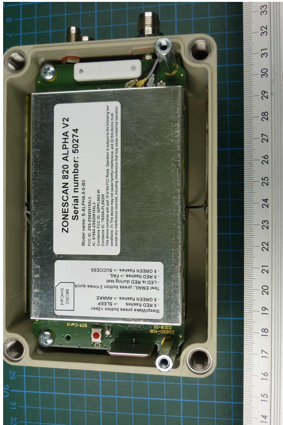
ZONESCAN 820 Alpha V2, internal view (FHSS antenna removed)
