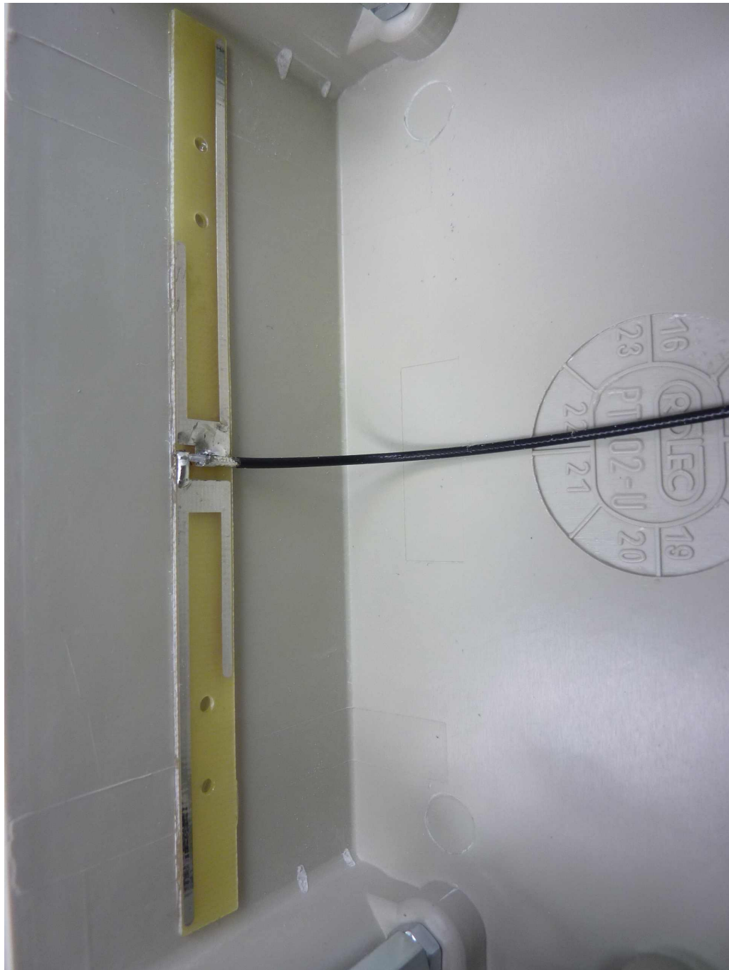
ZONESCAN 820 Alpha V2, internal view (detail view to cellular antenna)
