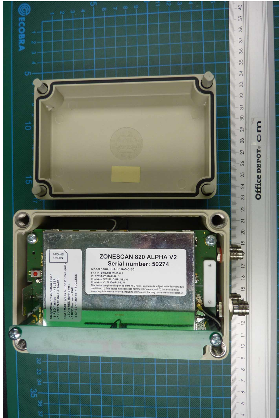
ZONESCAN 820 Alpha V2, internal view (housing opened)
