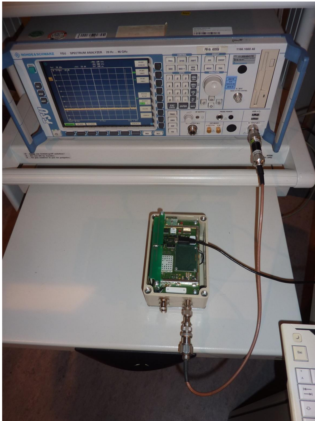
ZONSCAN 820 Alpha V2, test setup shielded chamber
