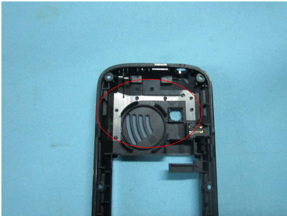
GSM Antenna View
