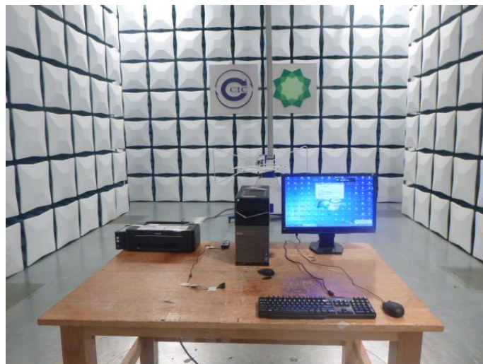
Radiated Emission (above 1GHz) Connect to PC
