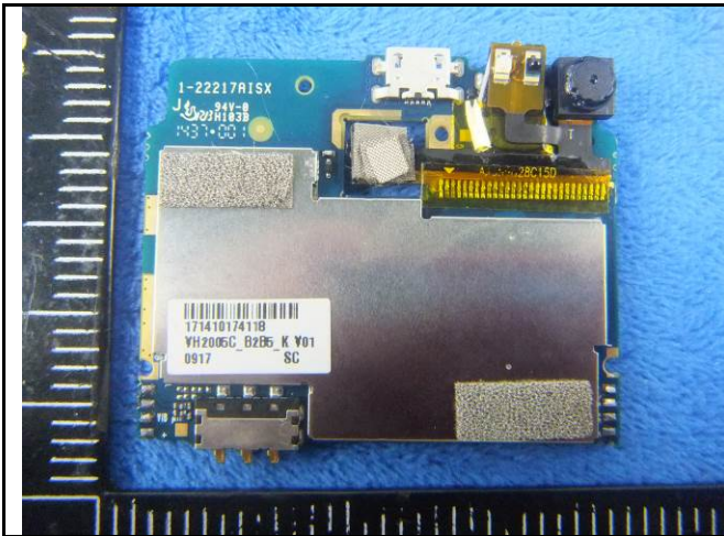
Mainborad With Shielding - Front View
