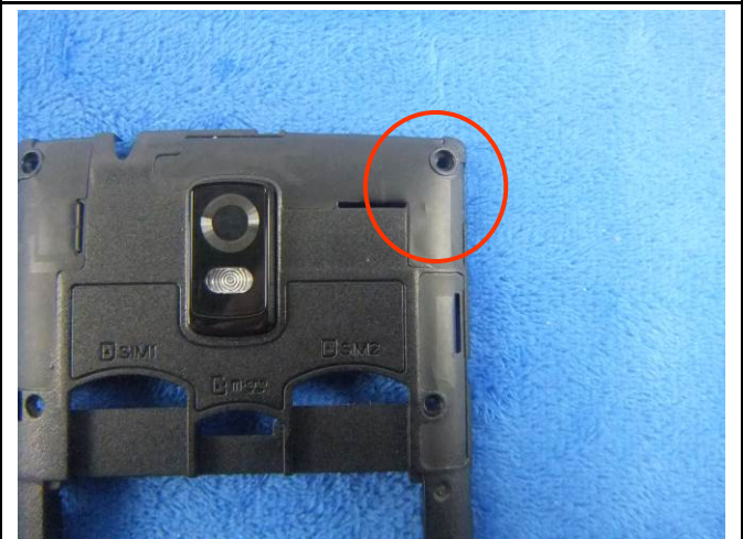
GSM/PCS/UMTS/ -FDD Antenna View
