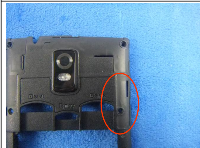
BT/WIFI Antenna View
