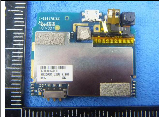
Mainborad With Shielding - Front View
