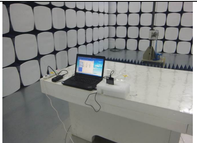
Radiated Spurious Emissions Test Setup Above 1GHz
