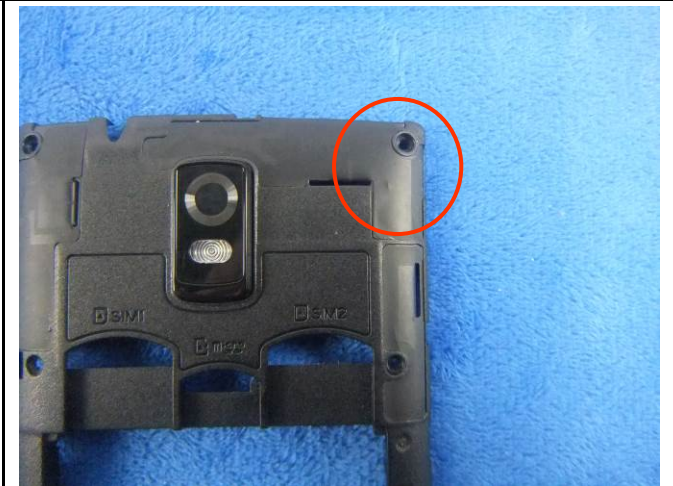
GSM/PCS/UMTS/-FDD Antenna View
