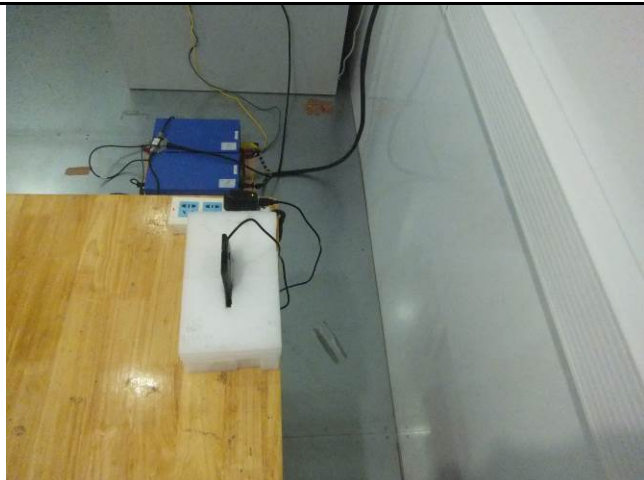
Conducted Emissions Test Setup Side View
