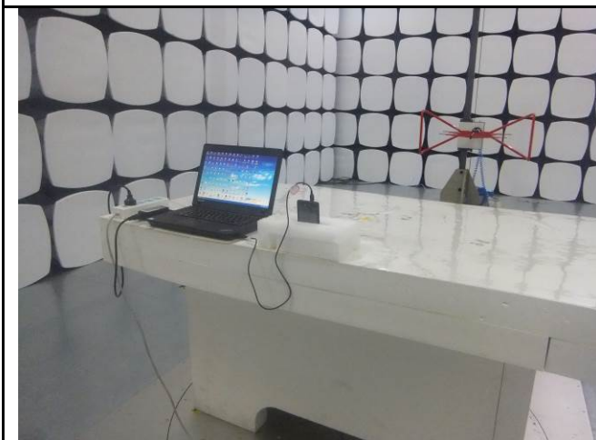
Conducted Emissions Test Setup – Front View
