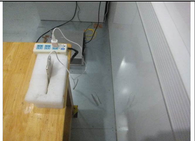
Conducted Emissions Test Setup Side View
