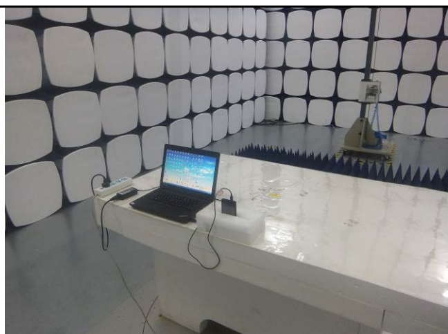
Radiated Spurious Emissions Test Setup Above 1GHz
