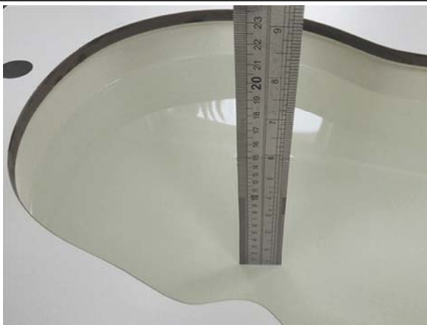
Liquid depth in the head phantom (2450MHz)
