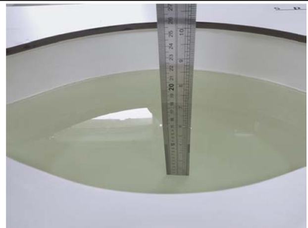
Liquid depth in the body phantom (2450MHz)
