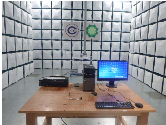
Radiated Emission (above 1GHz) Connect to PC
