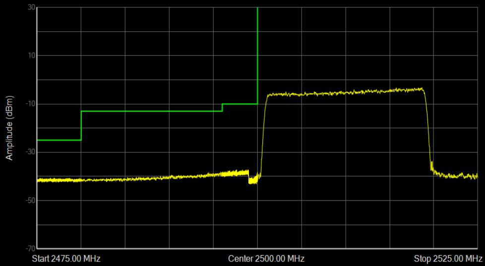
Band7 QAM16 BW=20MHz Channel=20850 RB Size=100 Position=#0
