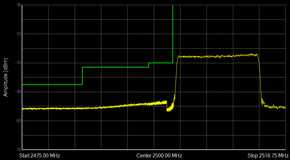
Band7 QAM16 BW=15MHz Channel=20825 RB Size=75 Position=#0
