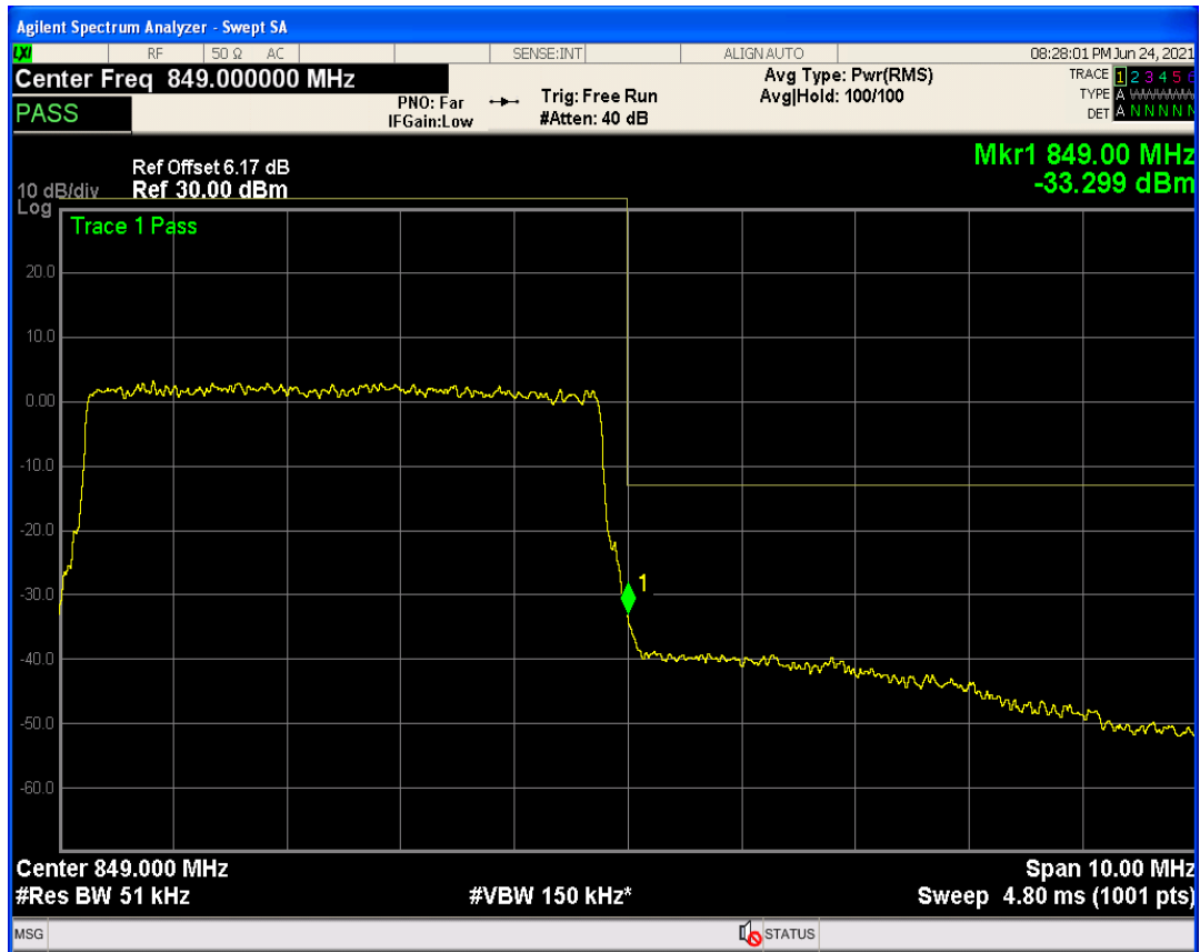
Band5 QAM16 BW=5MHz Channel=20625 RB Size=1 Position=#Max
