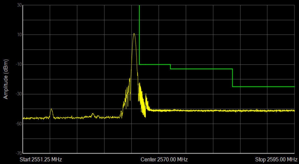
Band7 QAM16 BW=15MHz Channel=21375 RB Size=1 Position=#Max
