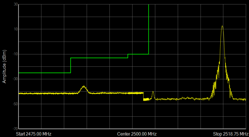
Band7 QPSK BW=15MHz Channel=20825 RB Size=1 Position=#Max
