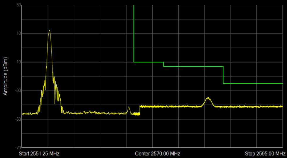
Band7 QPSK BW=15MHz Channel=21375 RB Size=1 Position=#0
