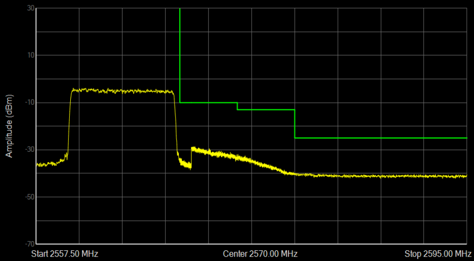
Band7 QPSK BW=10MHz Channel=21400 RB Size=50 Position=#0
