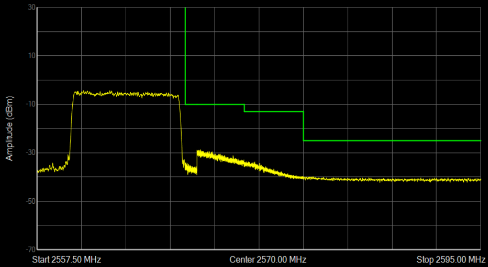
Band7 QAM16 BW=10MHz Channel=21400 RB Size=50 Position=#0
