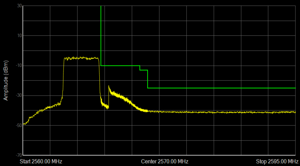
Band7 QPSK BW=5MHz Channel=21425 RB Size=25 Position=#0
