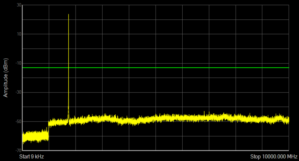
Band4 QAM16 BW=3MHz Channel=20385 RB Size=15 Position=#0
