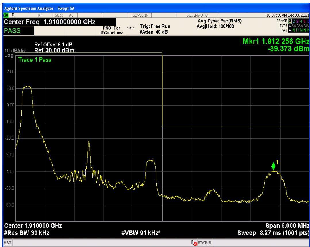
Band2 QAM16 BW=3MHz Channel=19185 RB Size=1 Position=#Max
