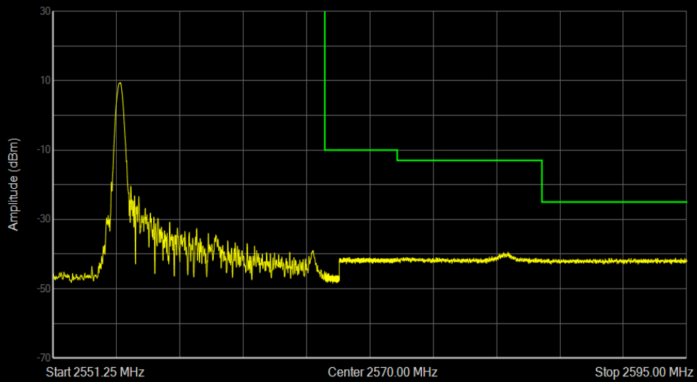
Band7 16QAM BW=15MHz Channel=21375 RB Size=1 Position=#0
