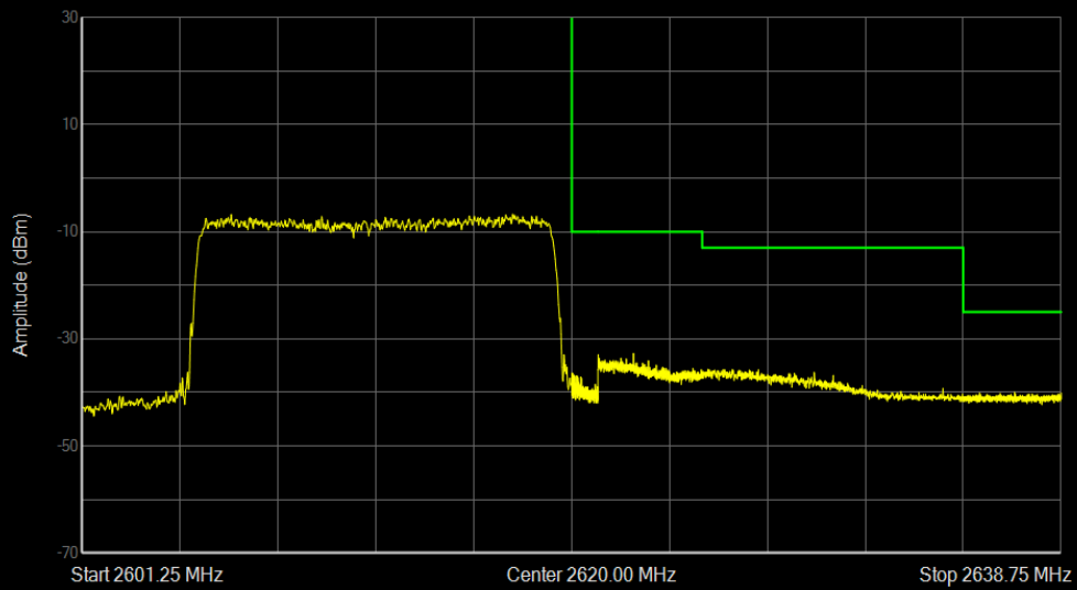
Band38 QPSK BW=15MHz Channel=38175 RB Size=75 Position=#0
