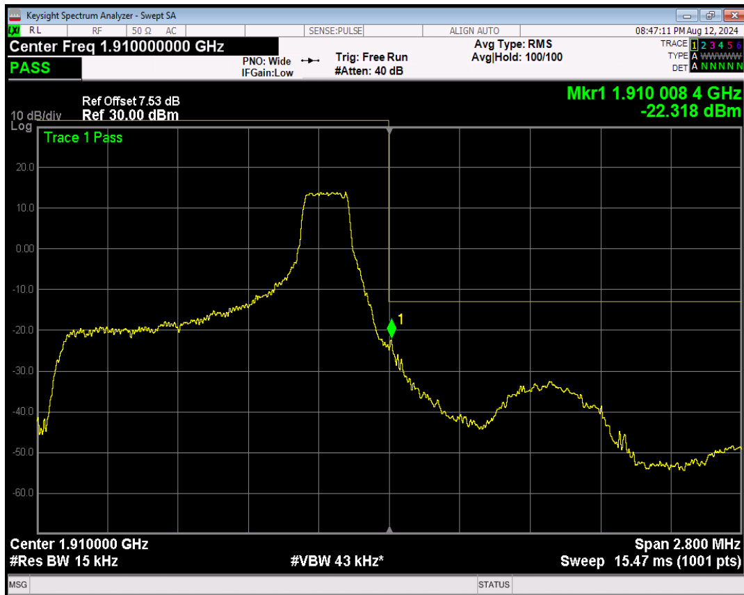
Band2 16QAM BW=1.4MHz Channel=19193 RB Size=6 Position=#0
