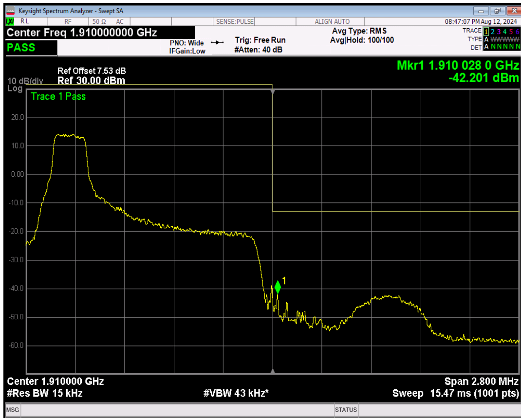
Band2 16QAM BW=1.4MHz Channel=19193 RB Size=1 Position=#Max
