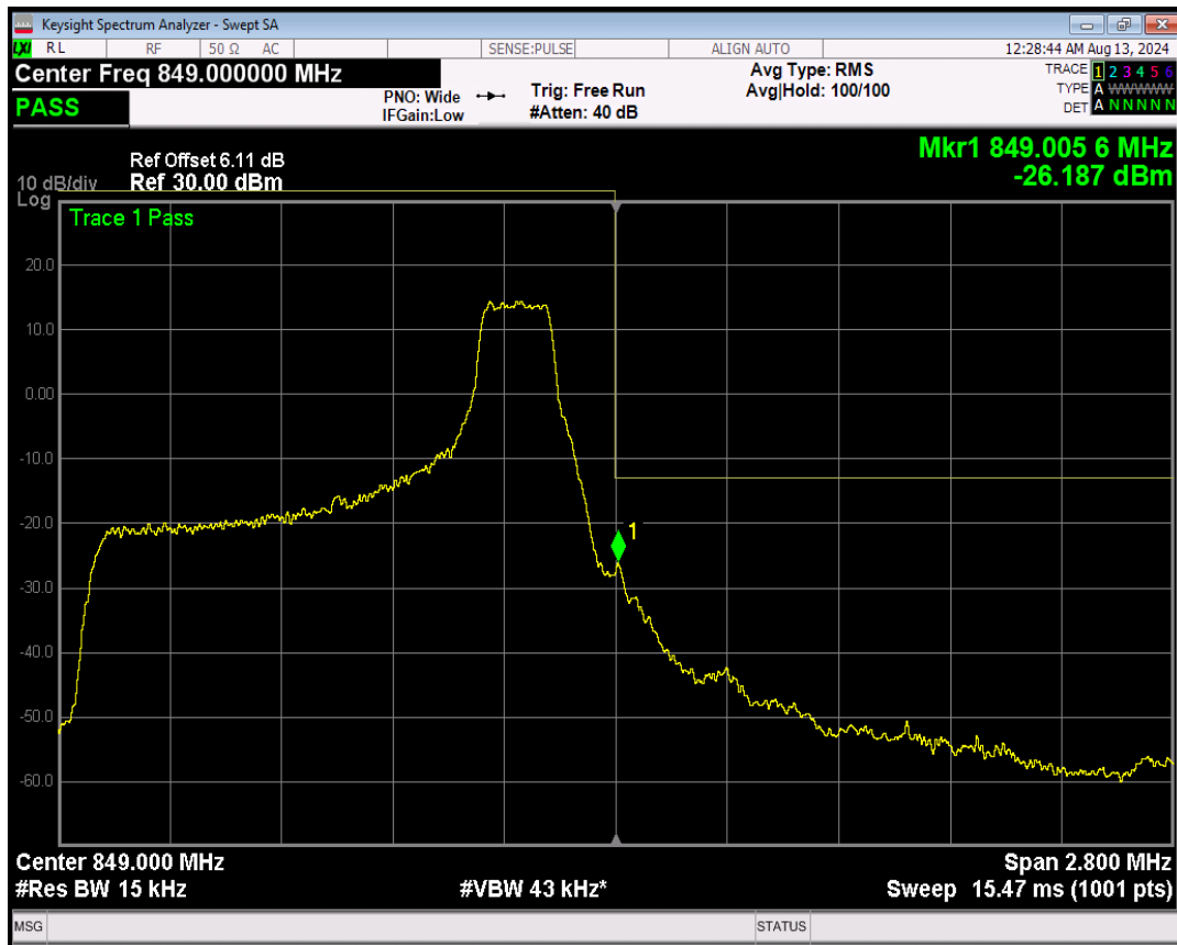
Band26(824-849) QPSK BW=1.4MHz Channel=27033 RB Size=6 Position=#0
