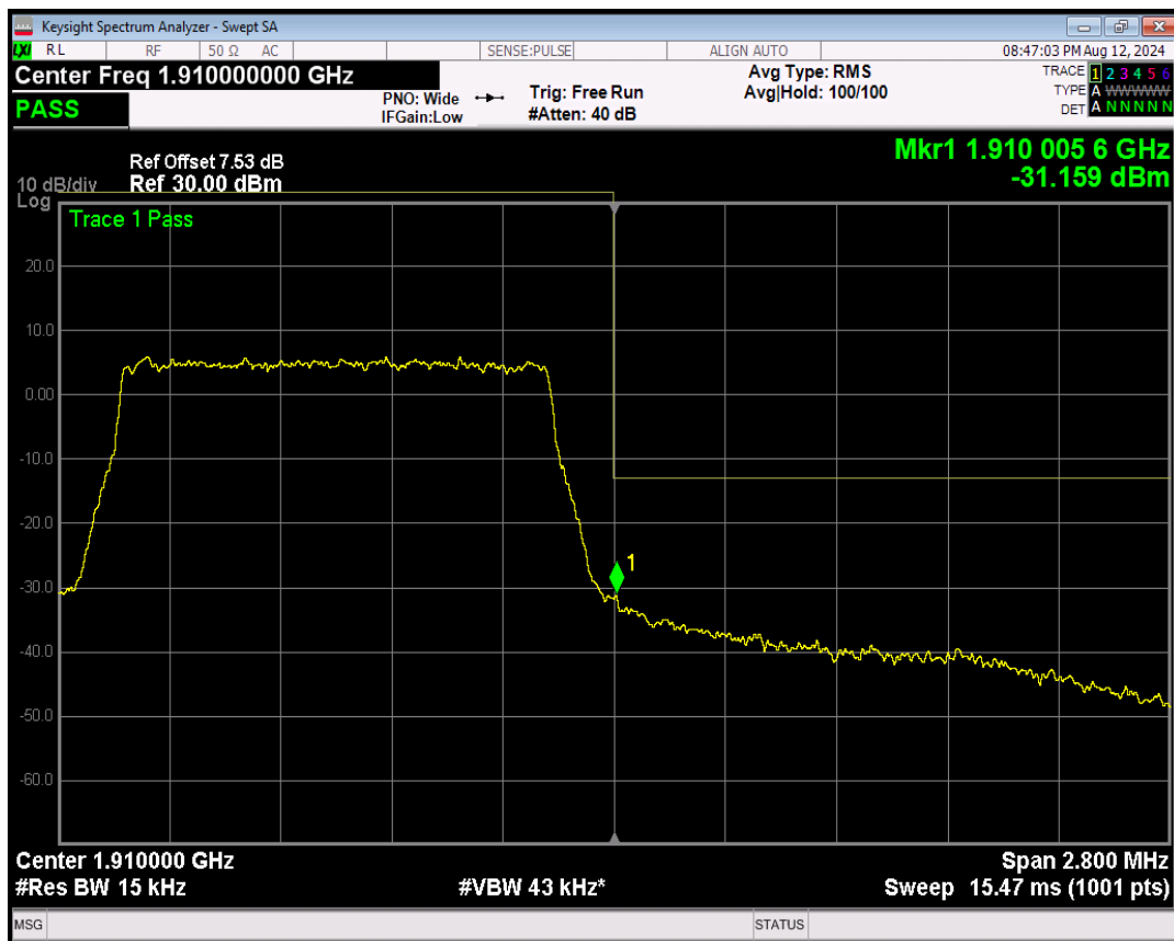
Band2 16QAM BW=1.4MHz Channel=19193 RB Size=1 Position=#0
