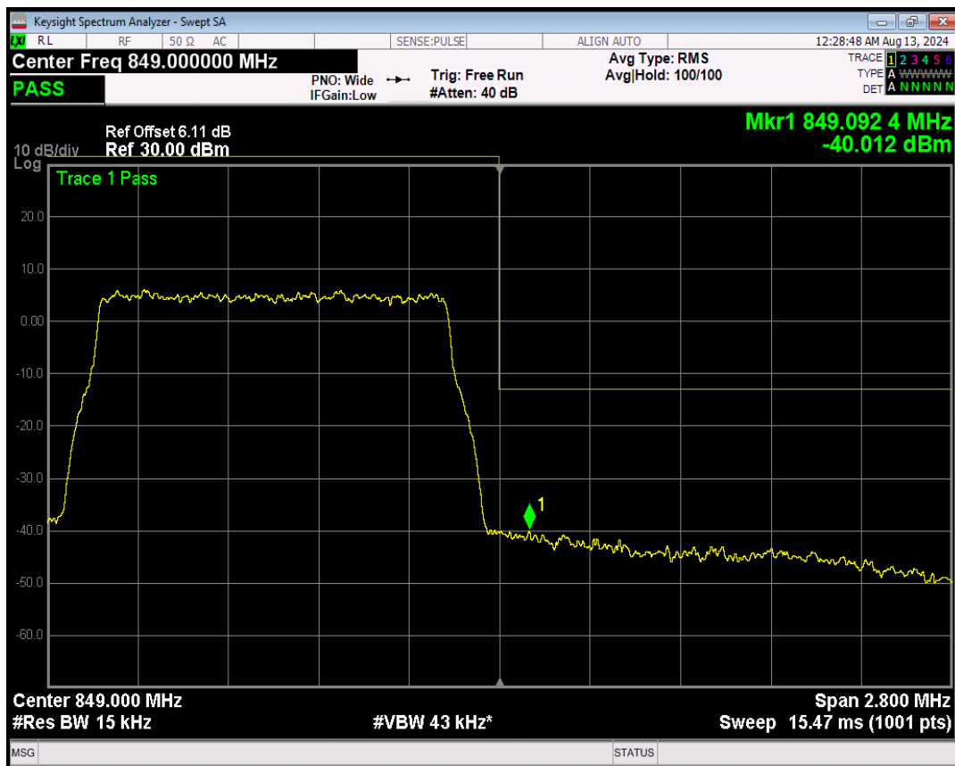
Band26(824-849) 16QAM BW=1.4MHz Channel=27033 RB Size=1 Position=#0
