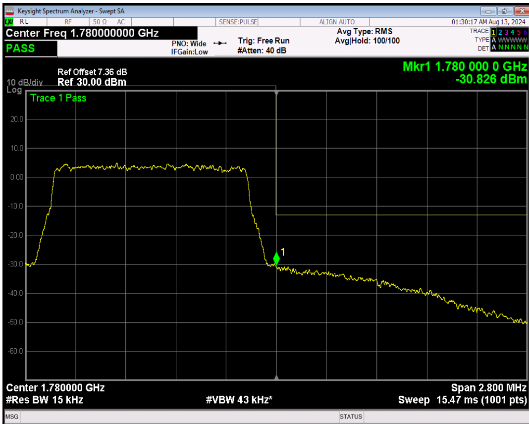
Band66 16QAM BW=1.4MHz Channel=132665 RB Size=1 Position=#0
