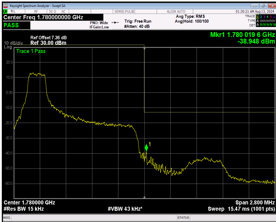
Band66 16QAM BW=1.4MHz Channel=132665 RB Size=1 Position=#Max
