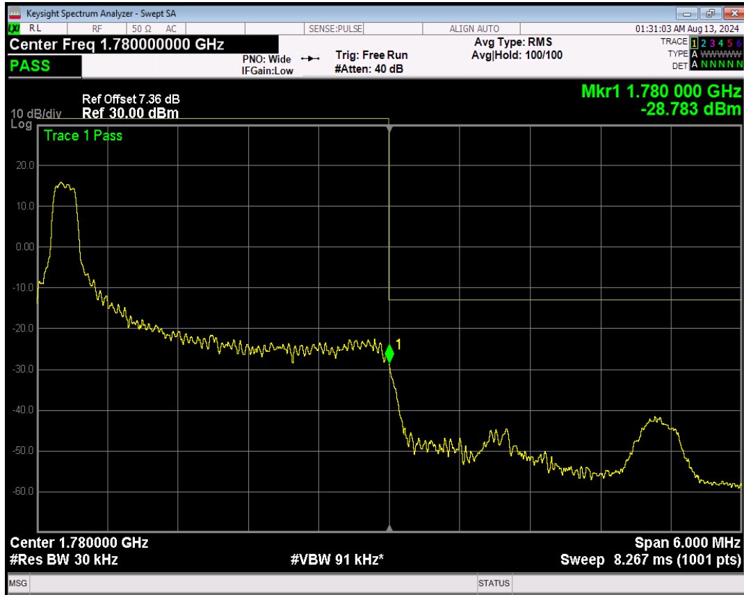
Band66 16QAM BW=3MHz Channel=132657 RB Size=1 Position=#Max
