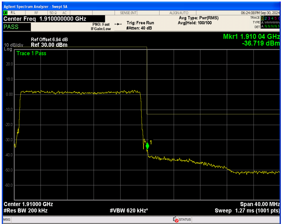
Band26a QPSK BW=1.4MHz Channel=26697 RB Size=1 Position=#0
