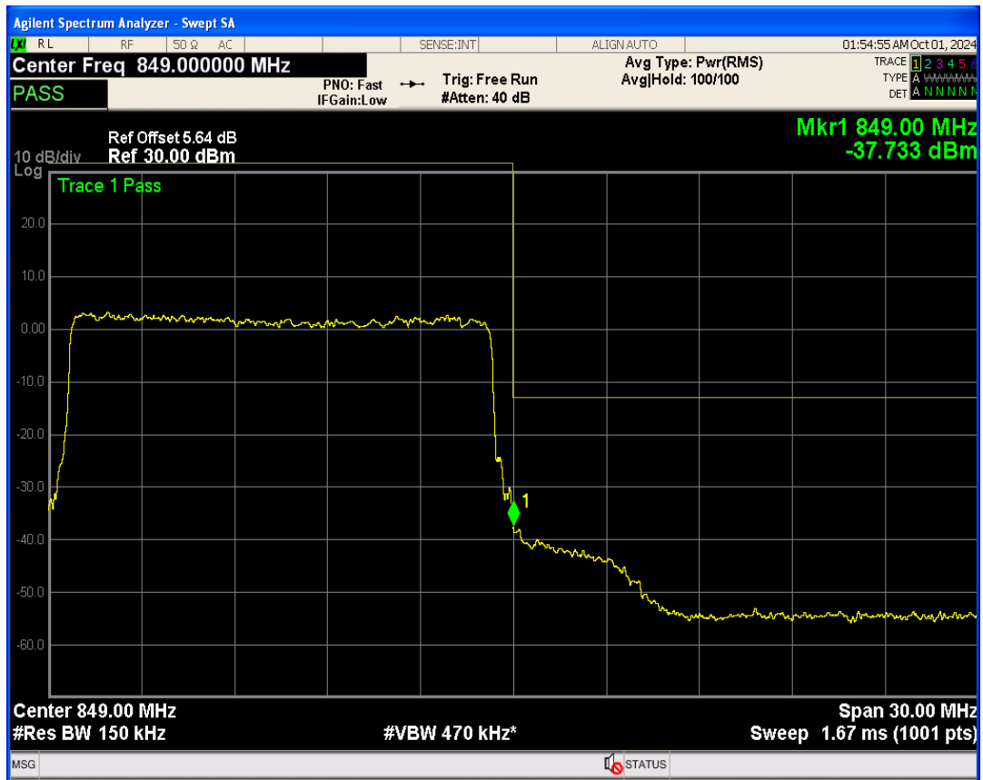
Band38 QPSK BW=5MHz Channel=37775 RB Size=1 Position=#0
