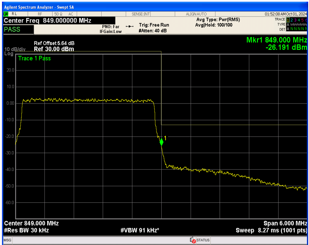
Band26b QPSK BW=5MHz Channel=26815 RB Size=1 Position=#Max
