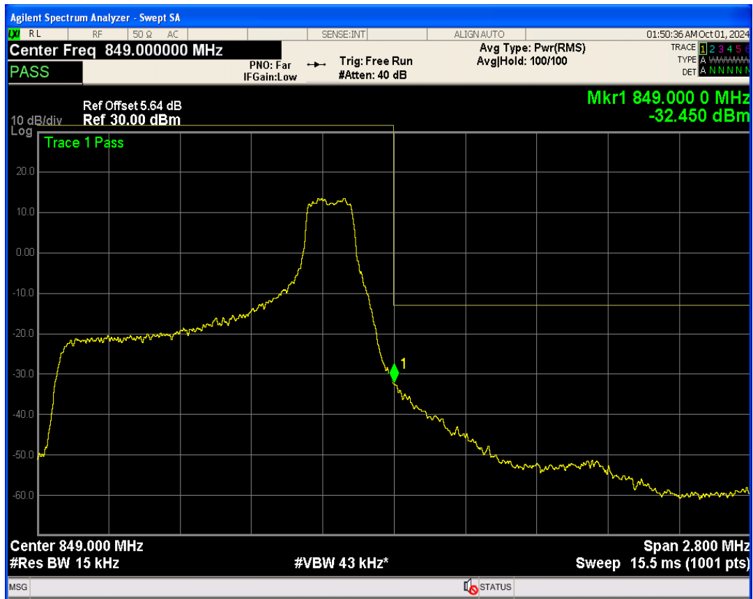
Band26b QPSK BW=1.4MHz Channel=27033 RB Size=6 Position=#0
