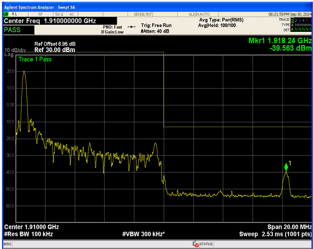
Band2 16QAM BW=10MHz Channel=19150 RB Size=1 Position=#Max
