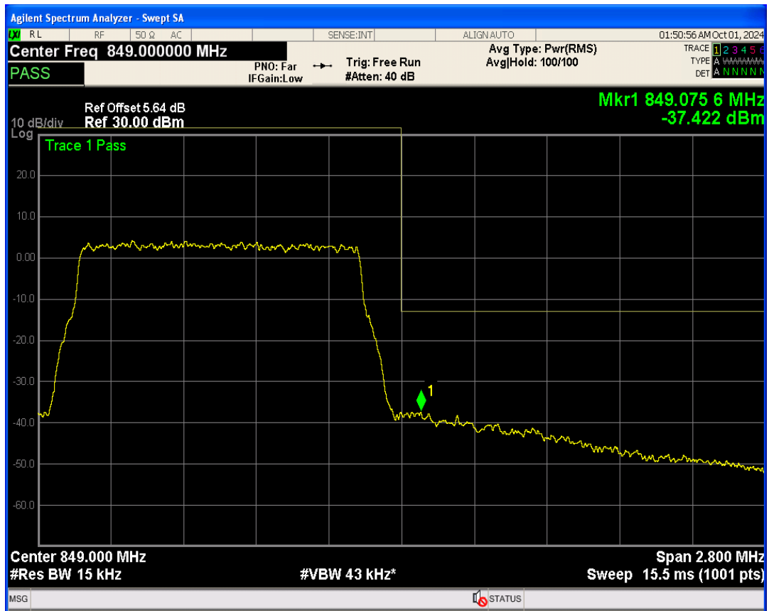
Band26b QPSK BW=3MHz Channel=26805 RB Size=1 Position=#Max
