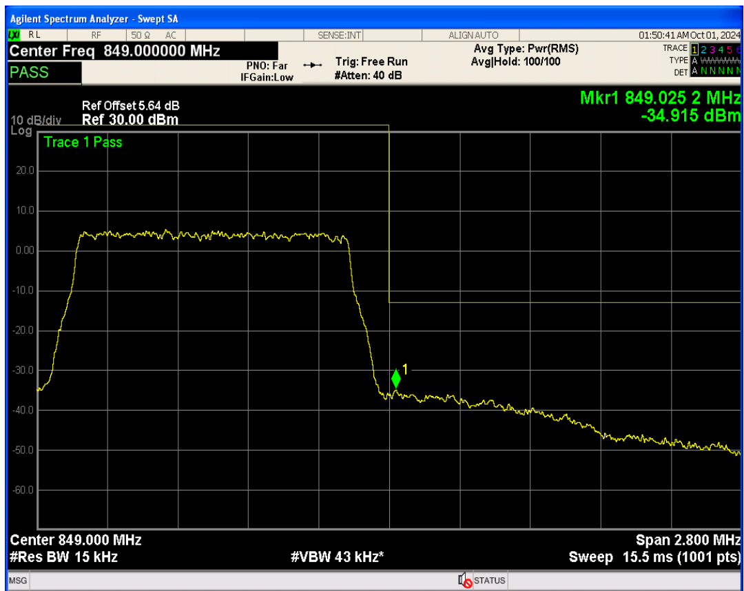
Band26b 16QAM BW=1.4MHz Channel=27033 RB Size=1 Position=#0
