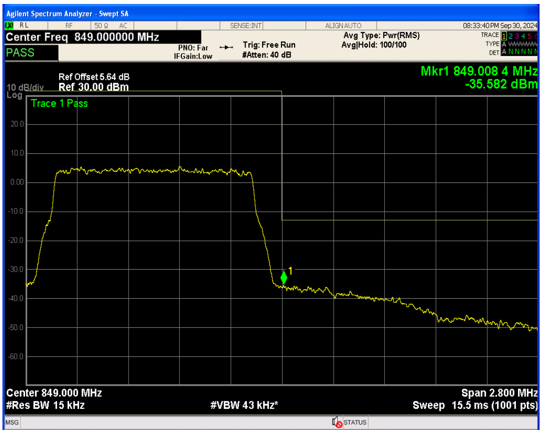
Band5 16QAM BW=1.4MHz Channel=20643 RB Size=1 Position=#0
