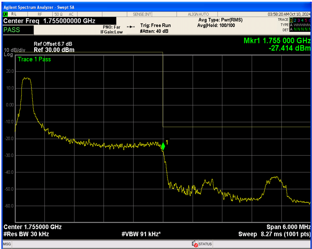
Band4 16QAM BW=3MHz Channel=20385 RB Size=15 Position=#0
