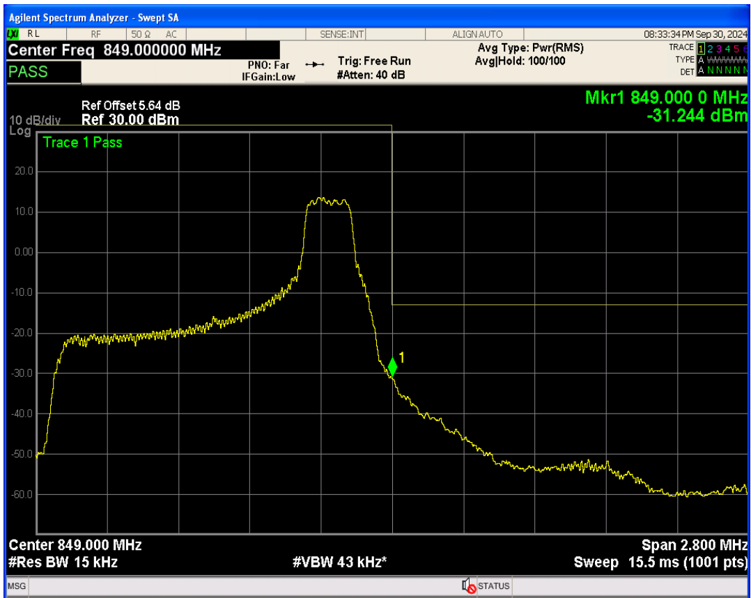
Band5 QPSK BW=1.4MHz Channel=20643 RB Size=6 Position=#0
