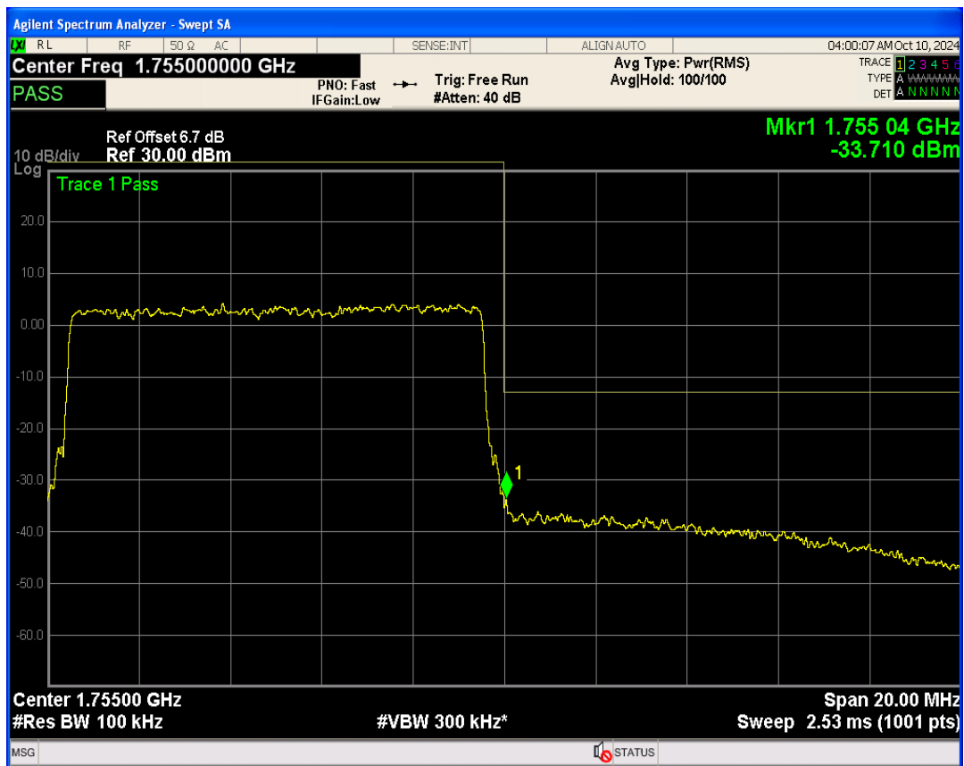
Band4 16QAM BW=10MHz Channel=20350 RB Size=1 Position=#0
