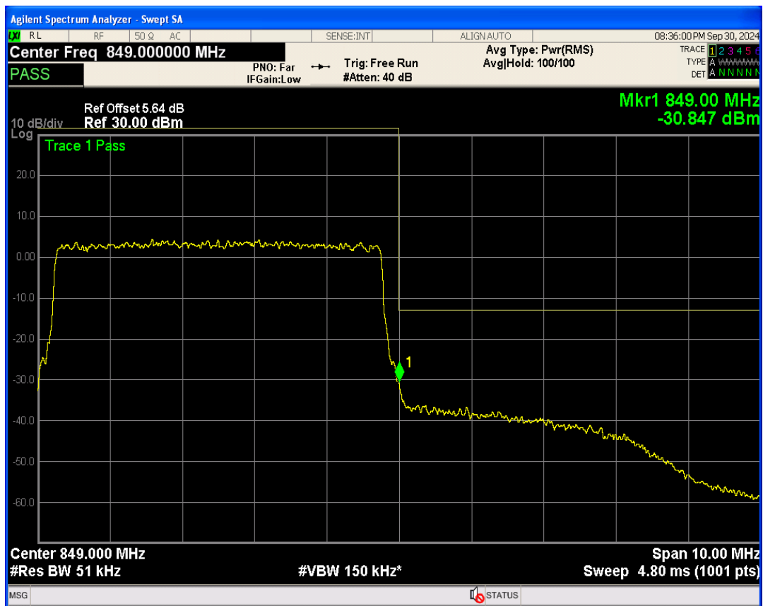
Band5 16QAM BW=5MHz Channel=20625 RB Size=1 Position=#0
