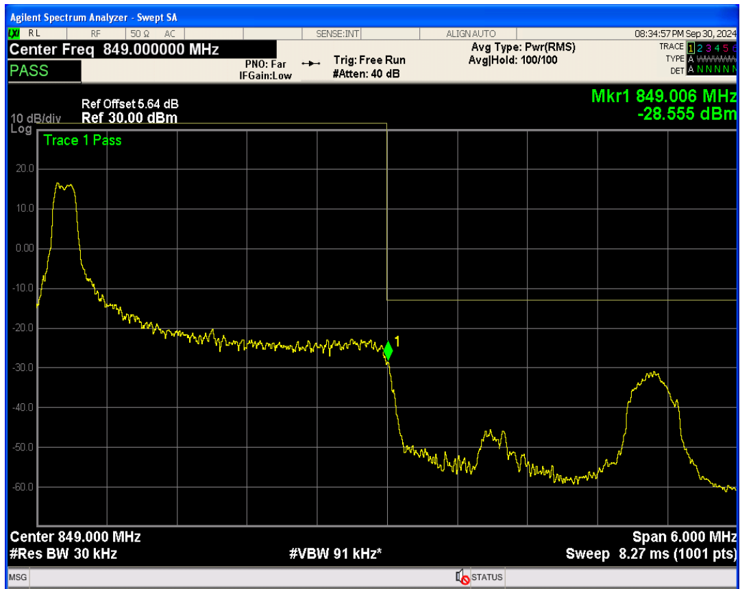
Band5 16QAM BW=3MHz Channel=20635 RB Size=1 Position=#Max
