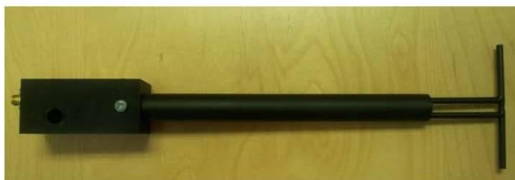
Figure 1 – MVG COMOSAR Validation Dipole
