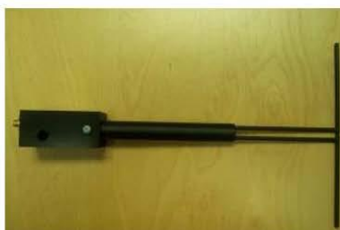
Figure 1 – MVG COMOSAR Validation Dipole
