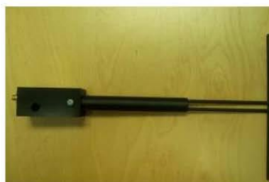
Figure 1 – MVG COMOSAR Validation Dipole
