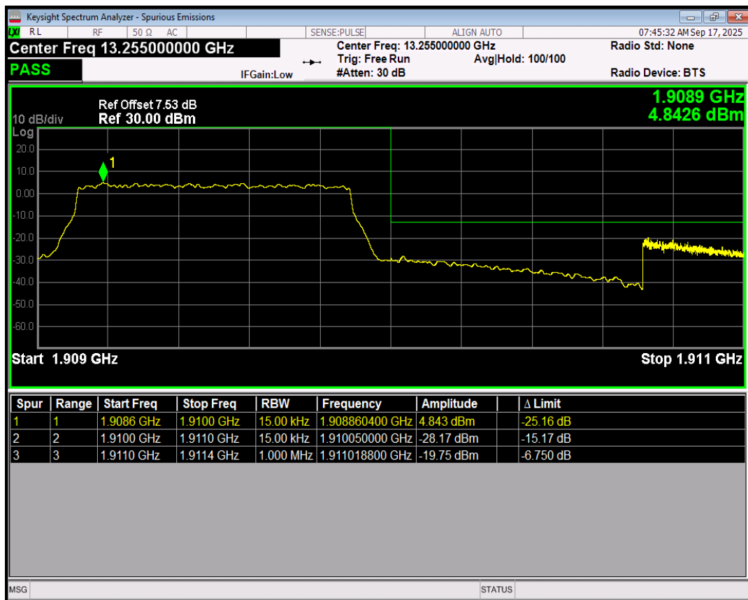
Band2 QPSK BW=3MHz Channel=18615 RB Size=1 Position=#0
