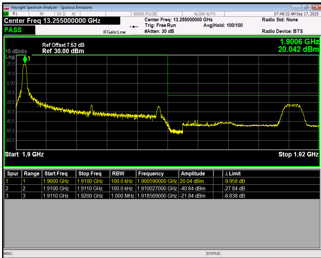
Band2 16QAM BW=10MHz Channel=19150 RB Size=1 Position=#Max
