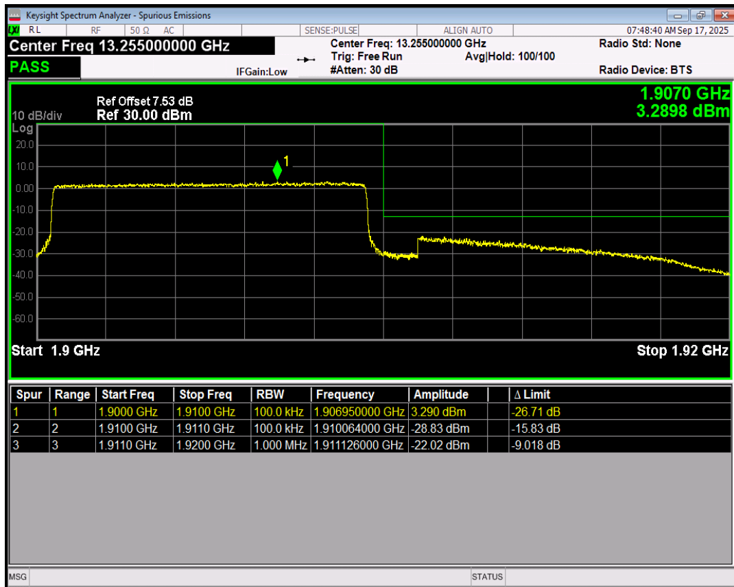
Band2 QPSK BW=15MHz Channel=18675 RB Size=1 Position=#0
