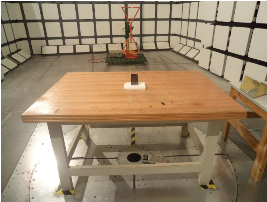
Radiated Emissions View (Below 1 GHz)
