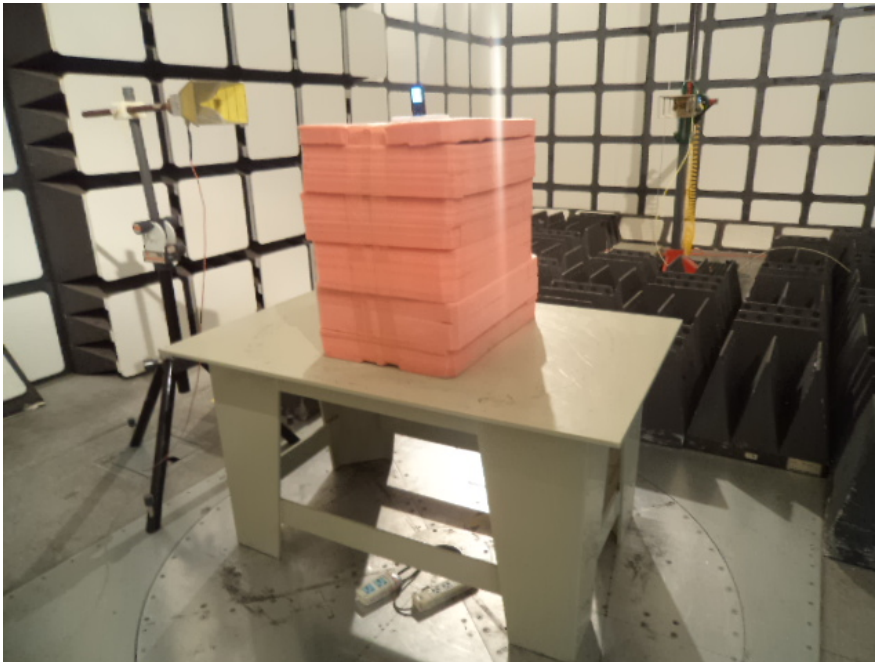
Radiated Emissions Test View (Above 1 GHz)
