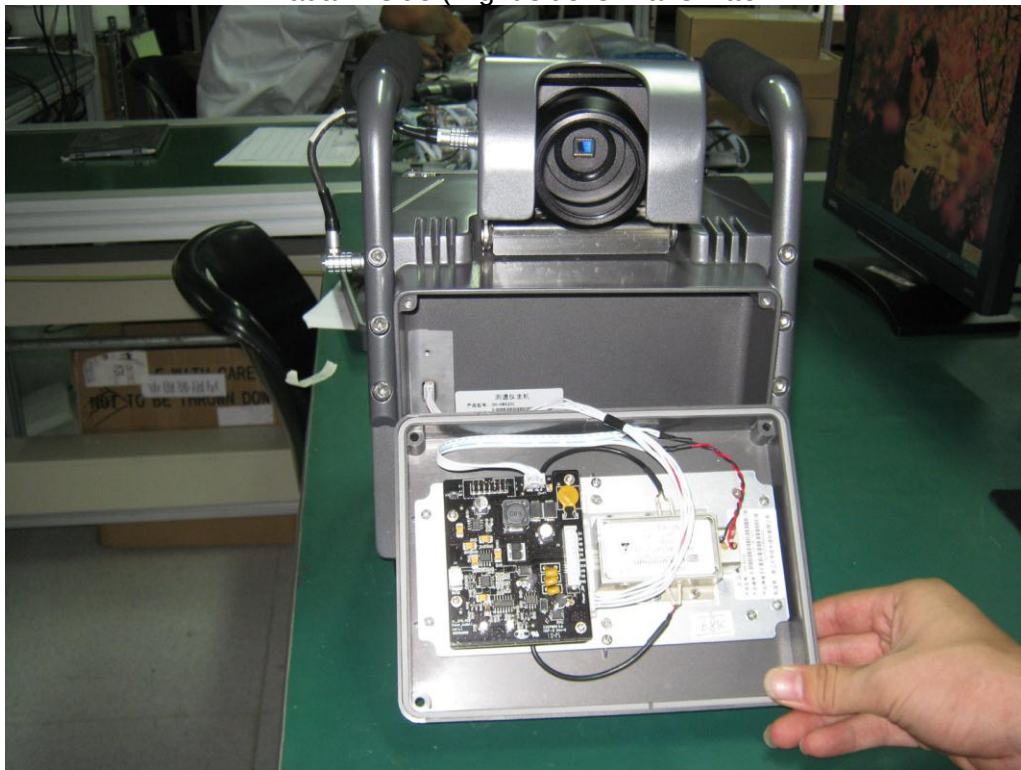
Radar Inside (Right side is Transmitter)
