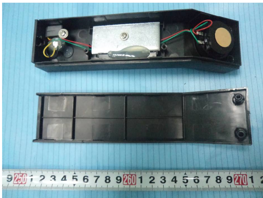
EUT (Handset) – Cover off View
