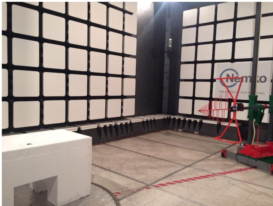
Figure 8.2-3: Emissions setup photo – 30 to 1000 MHz
