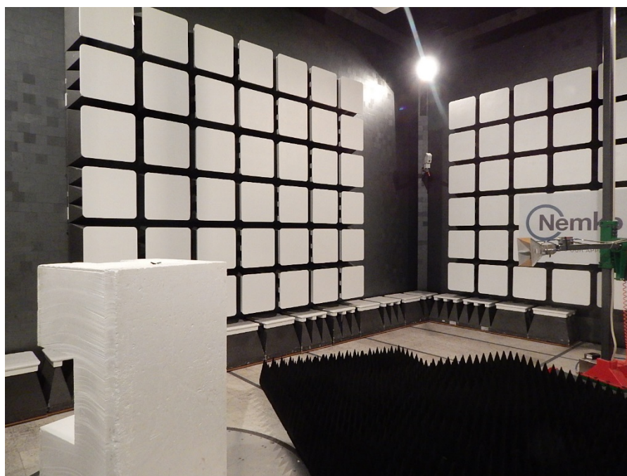
Figure 1-2: Emissions setup photo – above 1 GHz
