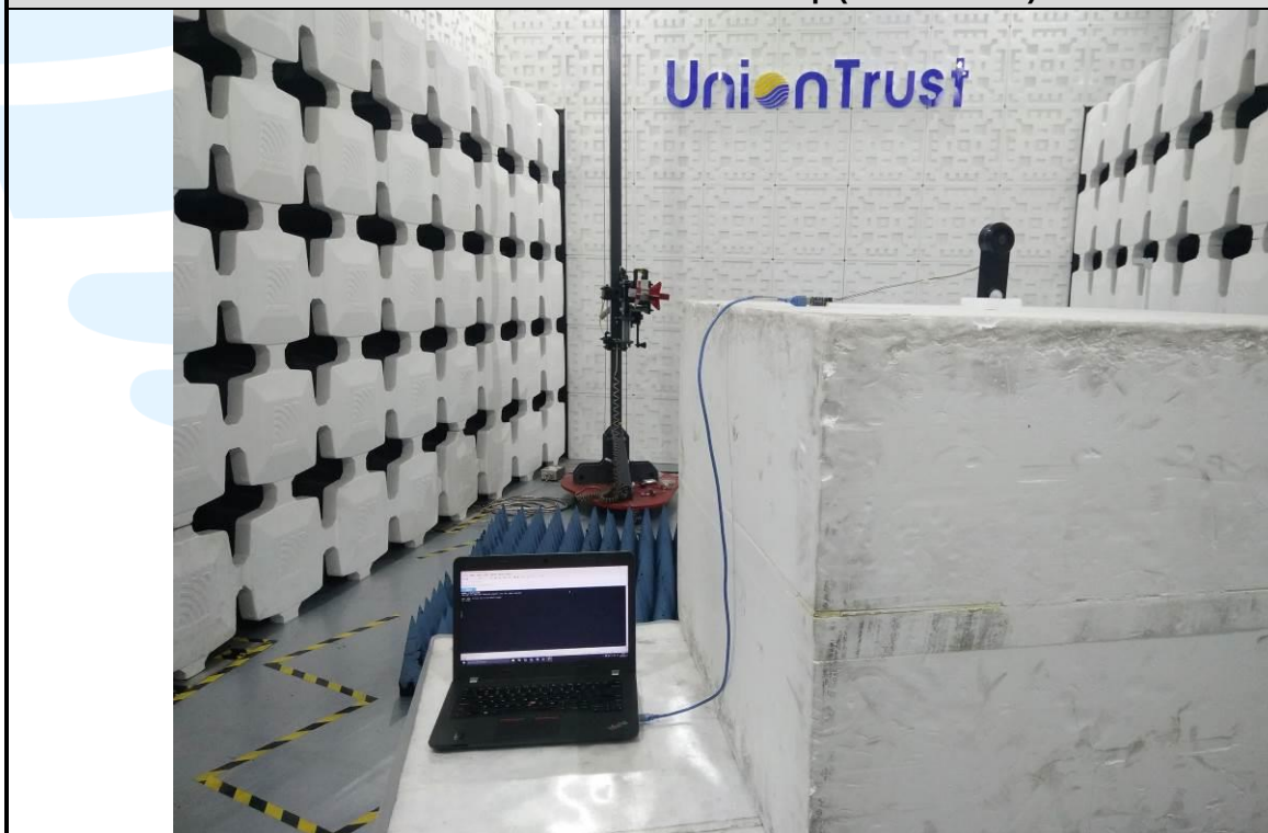
Radiated emission Test Setup (Above 1 GHz)
