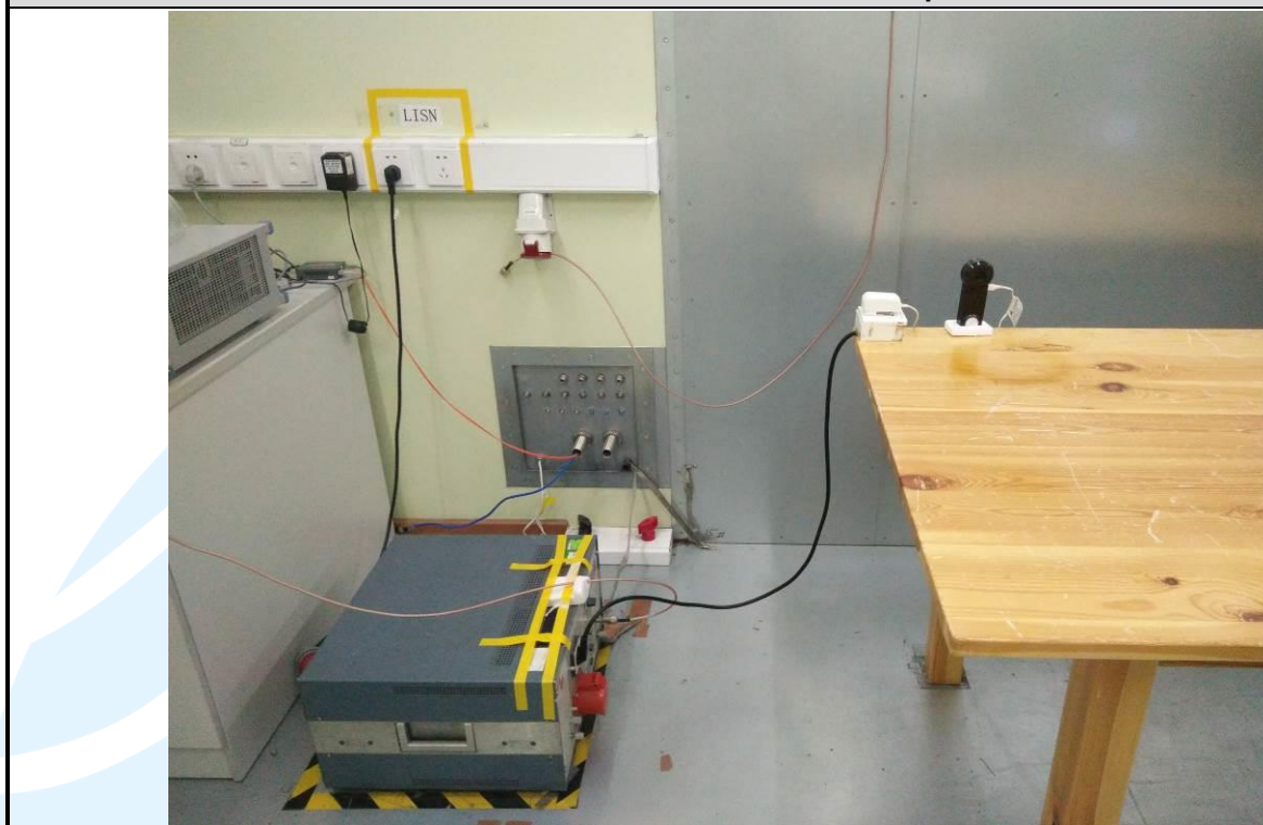
Conducted Emission Test Setup
