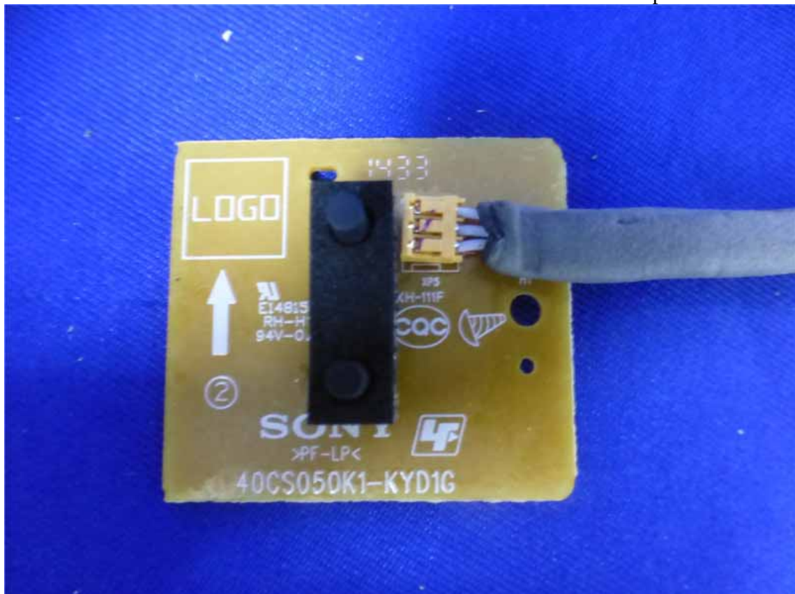
Figure 10 Components Side of the PCB
