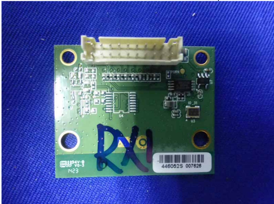
Figure 8 Components Side of the PCB
