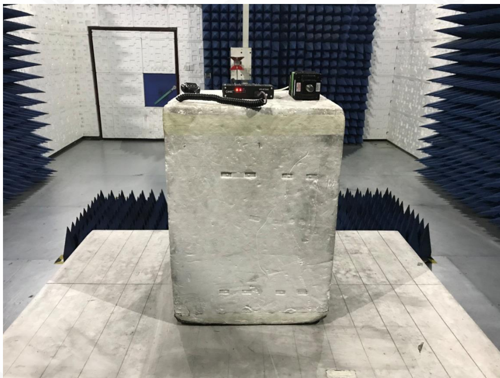
RADIATED EMISSION TEST SETUP ABOVE 1GHZ
