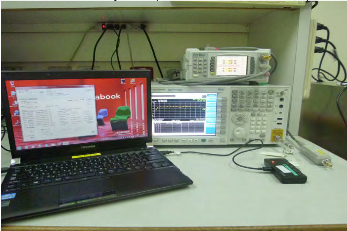
Conducted Setup Photo (Measurement at Antenna Port)
