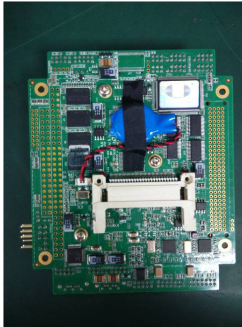
EUT –MCB Board Top Uncover View
