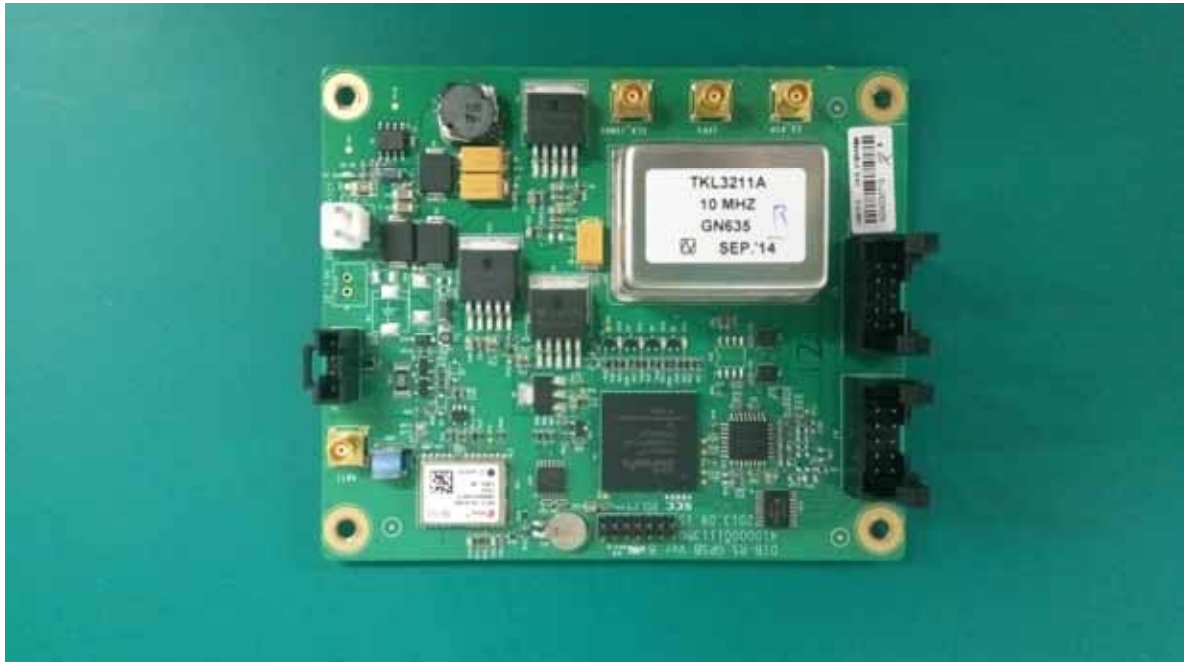
EUT –GNSS Board Top View
