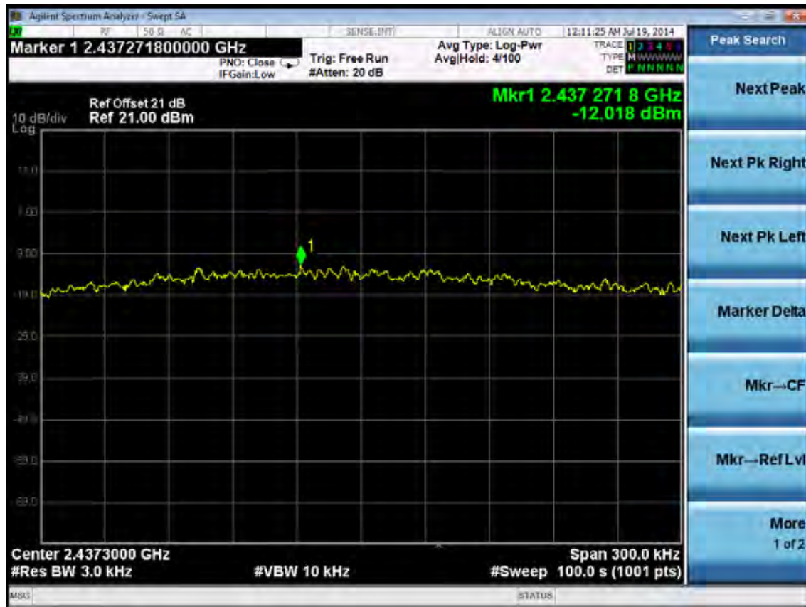
Test CH6: 2437MHz
