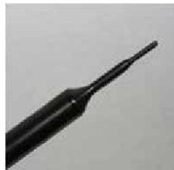
Figure 4.4 EX3DV4 E-field Probe
