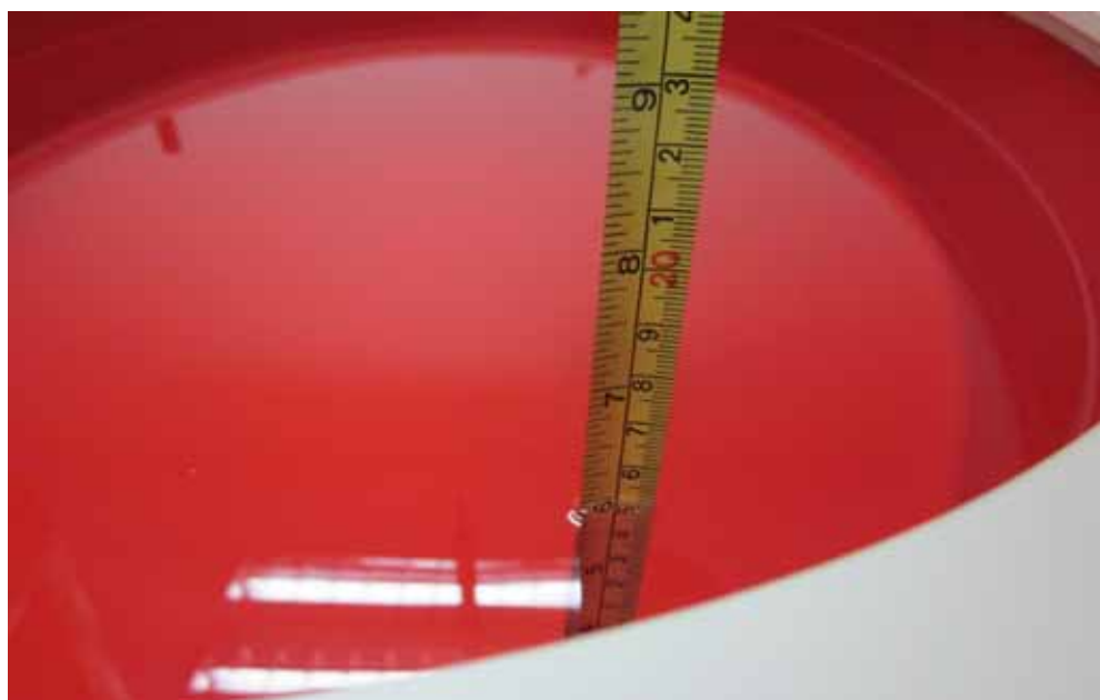
Figure 4.4: Liquid depth in the Flat Phantom
