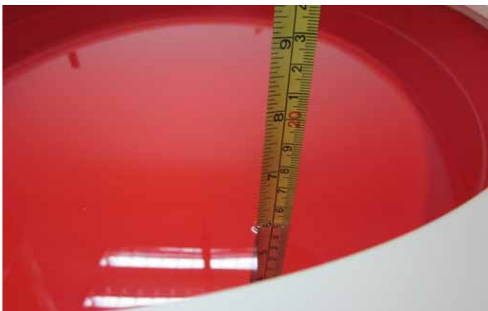
Figure 4.4: Liquid depth in the Flat Phantom
