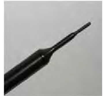
Figure 4.4 EX3DV4 E-field Probe
